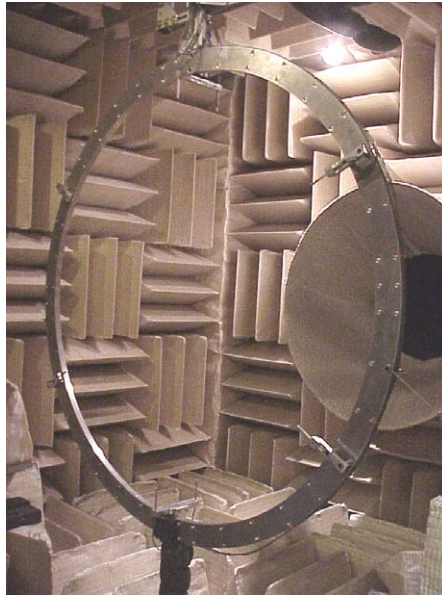
Fig. 4. Photograph of the arc array in the anechoic chamber. For actual data acquisition, the ring was wrapped in acoustic foam.
